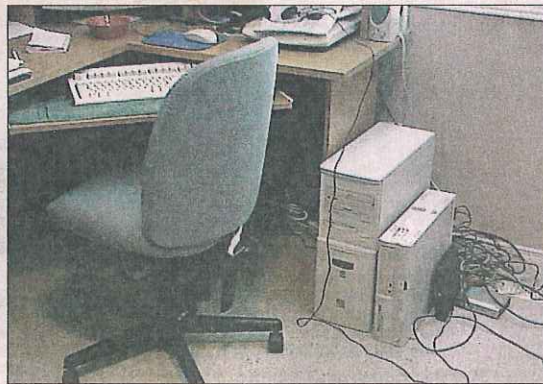
This maze of cables can be untangled, then neatly bundled with wire ties.
